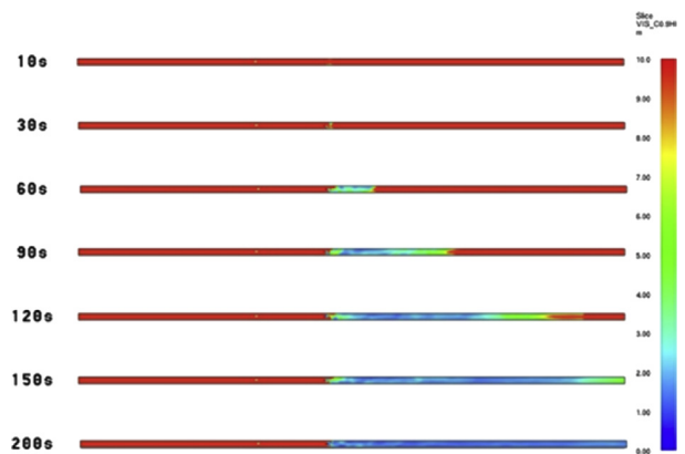
Fig. 14. Vision contour at 2 m above the tunnel floor in the presence of the jet fan.
