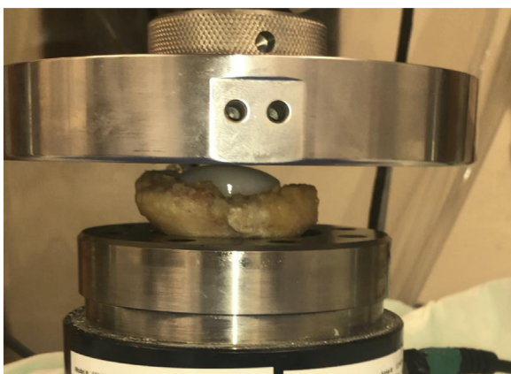
Figure 3. Compression plate attached to the actuator descending at a rate of 5 mm/s in axial compression until ultimate load to failure representing a patella fracture occurred.
