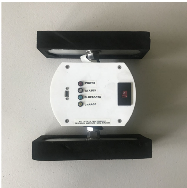
FIGURE 2 In-house strain gauge device for assessing hip adductor strength.
