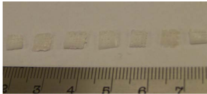
Figure 7. Photograph of PCL scaffolds eroded in 5 M NaOH medium at 55 °C at t = 0, 5, 20, 25, 30, 35, and 40 h.
