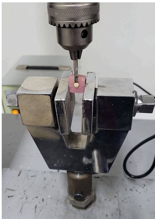
Fig. 3. Shows shear stress measurement device used in this study.
