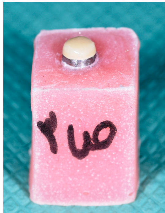
Fig. 2. Placing disc in an acrylic block for ease of use during shear stress measurement.
