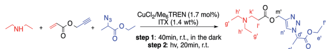
Scheme 2 One-pot, two-step sequential click reactions with propargyl acrylate, diethylamine and ethyl 2-azidopropionate (1/1/1 molar ratio). Irradiation conditions: Hg-Xe lamp filtered with borosilicate glass, 180 mW cm -2 and 20 min at room temperature.
