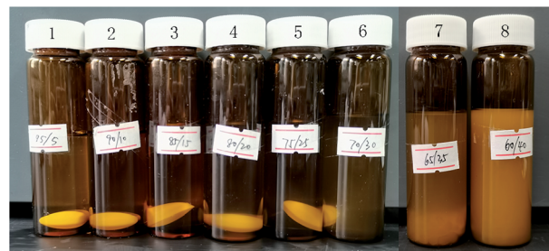
Fig. 1 The mixtures of 10 wt% PLA in different mass ratios of chloroform/ethanol mixed solutions (numbers 1 to 8 represent chloroform/ethanol = 95/5, 90/10, 85/15, 80/20, 75/25, 70/30, 65/35, 60/40 wt%, respectively).
