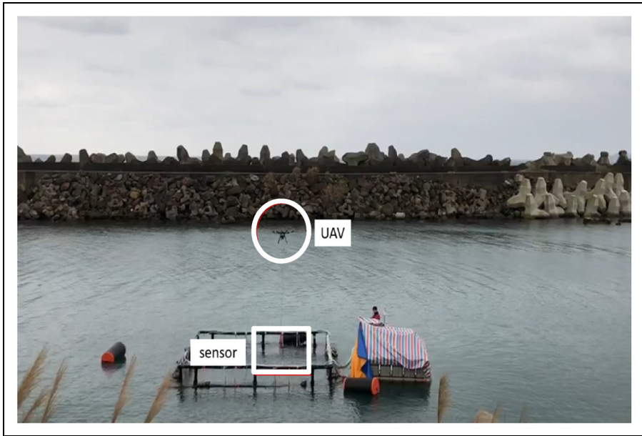
Figure 35. Dropping the sensor into the net cage.
