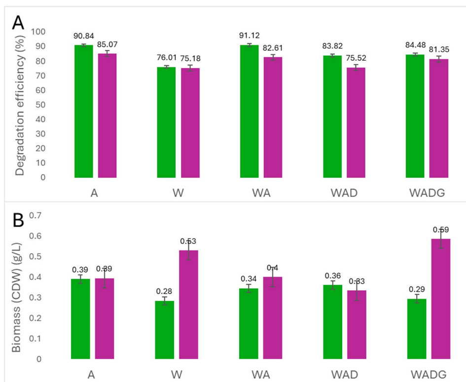
Fig. 2 A – Feather degradation efficiency for microbial hydrolysis of feather materials. The feathers were pretreated by autoclaving (A), washing (W), washing and autoclaving (WA), washing, autoclaving and drying (WAD), and washing, autoclaving, drying, and grinding (WADG). The results are shown for 5 days of growth of B. licheniformis (green) and 7 days of growth of A. oryzae (purple). B – Bacterial biomass (cell dry weight (CDW)) obtained after 5 and 7 days of bacterial hydrolysis, respectively, for B. licheniformis and A. oryzae . The standard deviation was calculated between the biological triplicates of the produced hydrolysates
