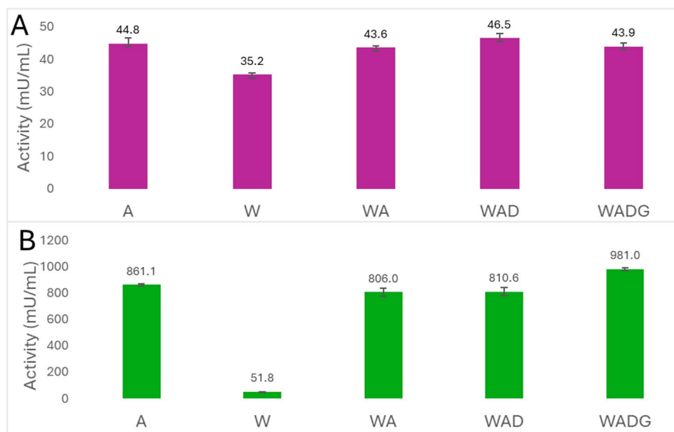
Fig. 3 Non-specific proteolytic activity in culture supernatant of hydrolysate samples. The feathers were pretreated by autoclaving (A), washing (W), washing and autoclaving (WA), washing, autoclaving and drying (WAD), and washing, autoclaving, drying and grinding (WADG). The results are shown for A : 7 days growth of A. oryzae and B : 5 days growth of B. licheniformis . The standard deviation was calculated between the biological and technical triplicates. Note the scale difference in the y axis
