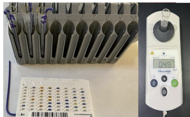
Fig. 4. Bacterial identification using the VITEK 2 Compact system and adjusting the turbidity of the solution of S. aureus using a turbidimeter.
