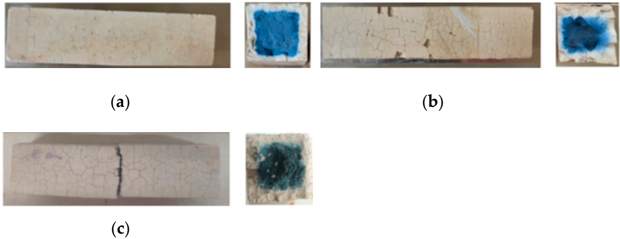
Figure 3. The surface of specimens after water W-D cycles. (a) SH 150 cycles (b) SS 150 cycles (c) SSG 20 cycles. used than the SH, and the colour of the blue substance was relatively lighter. Some of the SSG specimens began to break into two sections along the cracks at 20 cycles, and this section also showed that the surrounding blue geopolymer turned white.
