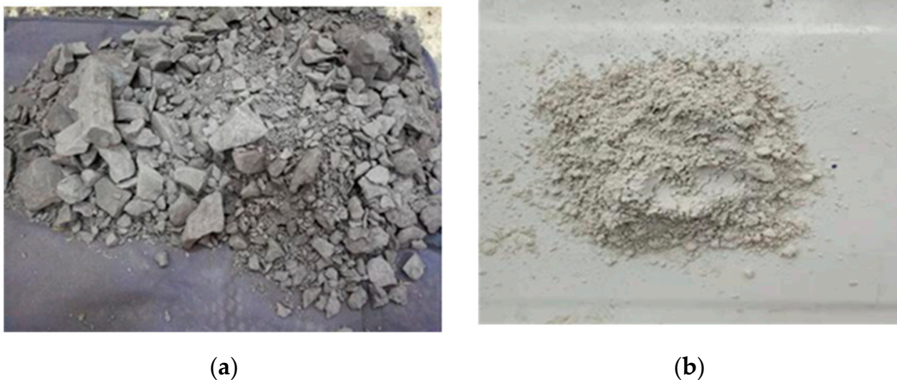
Figure 1. Raw materials. (a) Raw coal gangue; (b) Slag.
