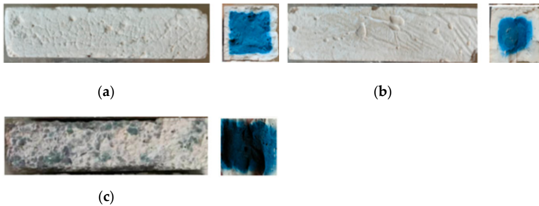
Figure 5. Surface and cross-sectional view of the specimens after sulphate W-D cycles. (a) SH 150 cycles (b) SS 150 cycles (c) SSG 3 cycles.
