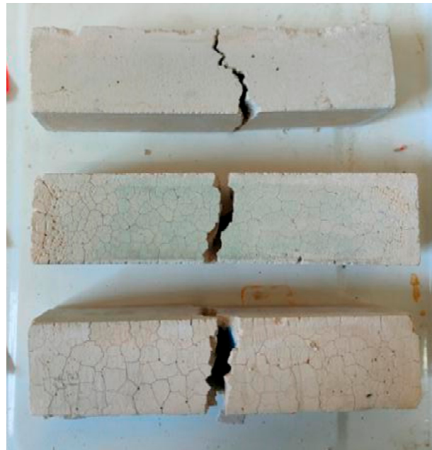
Figure 9. Specimen damaged in flexural test.
