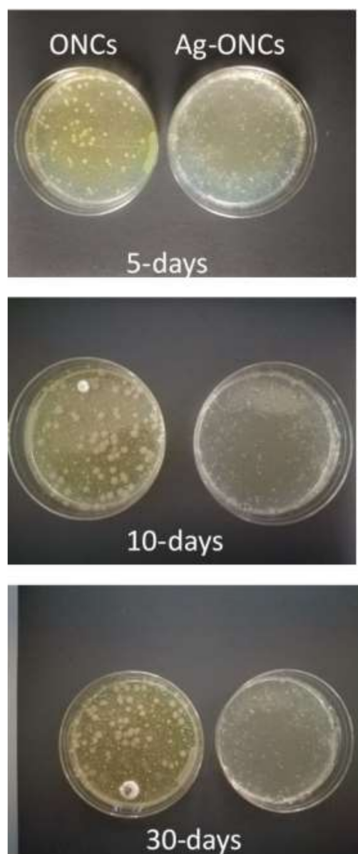
Figure 5. Comparison between ONCs and Ag-ONCs' antibacterial properties after different incubation times. Petri dishes are stored at room temperature under natural light.
