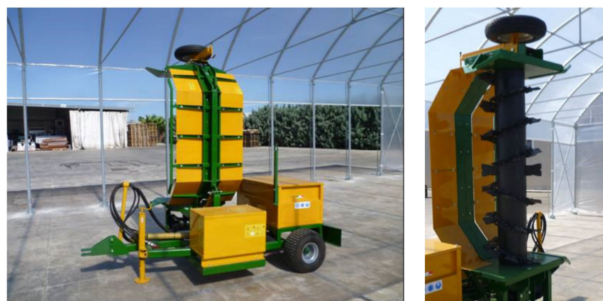
Figure 2. Turner machine (left); detail of the rotating shaft (right).
