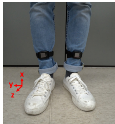
Figure 1. Gait measurements by two inertial measurement units (IMUs).
