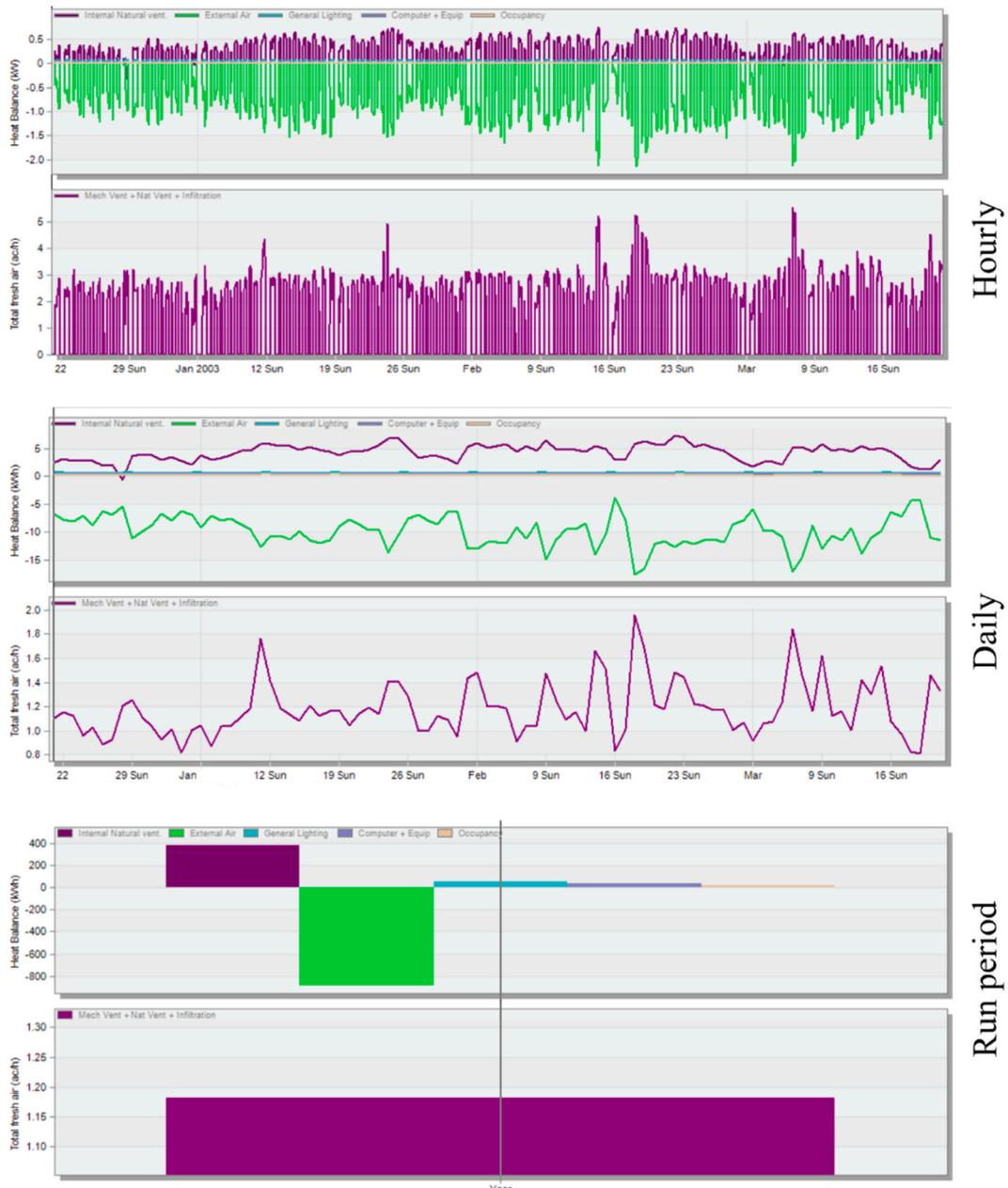
Fig. 6. Air change per hour calculations of the base case.
