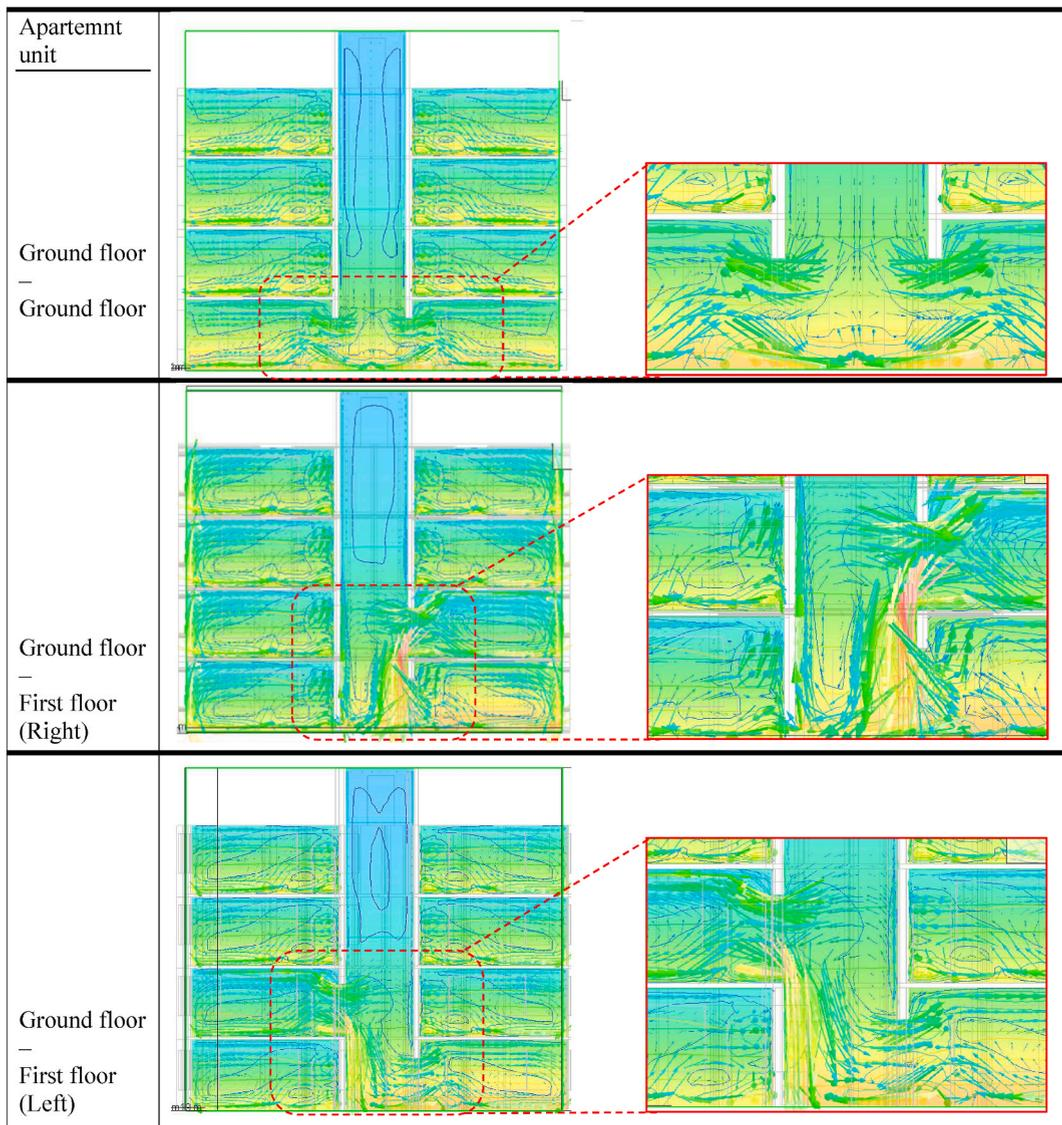
Fig. 11. CFD analysis of airflow exchange between different apartment units.
