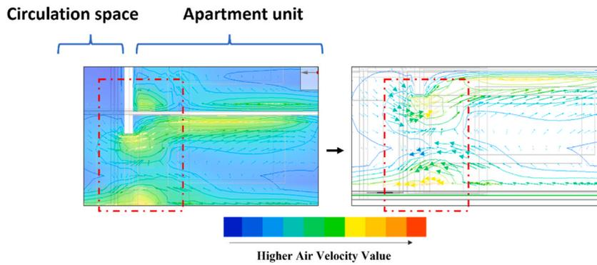
Fig. 10. Airflow exchange CFD analysis between an apartment unit and the common vertical circulation space.
