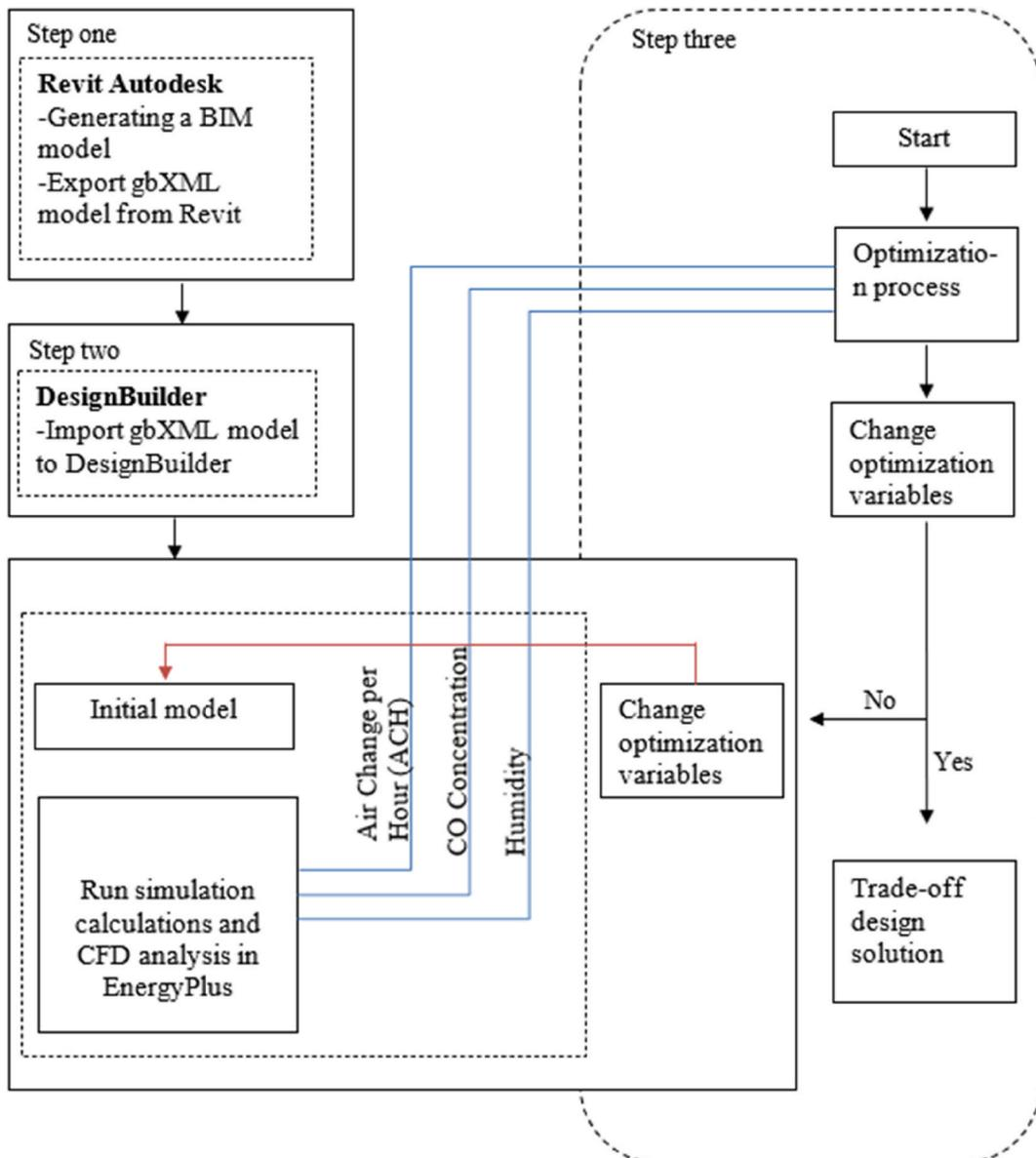
Fig. 1. Simulation and CFD analysis framework.
