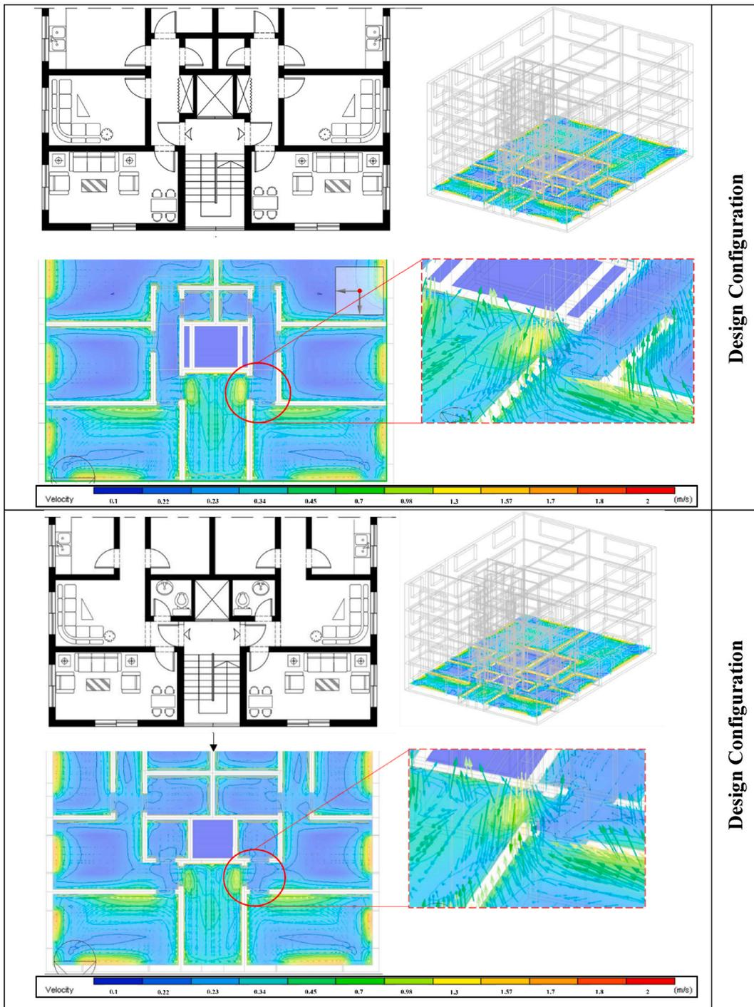
Fig. 12. Airflow into apartment units with different entryway design configurations.
