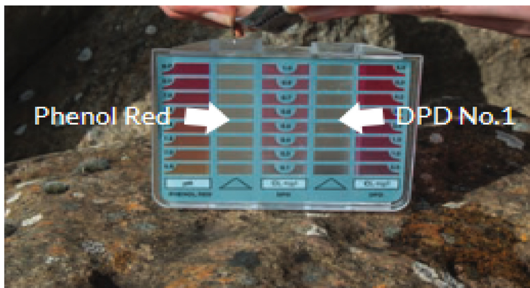
Figure 2. Color comparator device for free chlorine residual and pH determination. Taken from [18].
