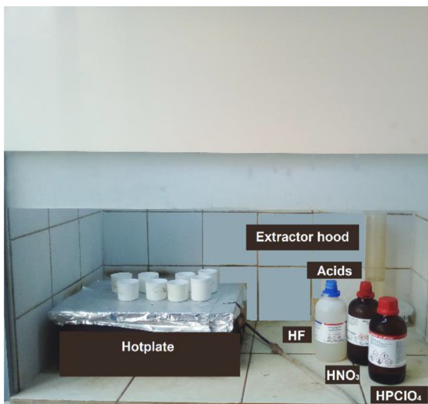
Figure 4. A photo showing the experimental tools that were used for the acid attack that was carried out on soil samples in the laboratory.
