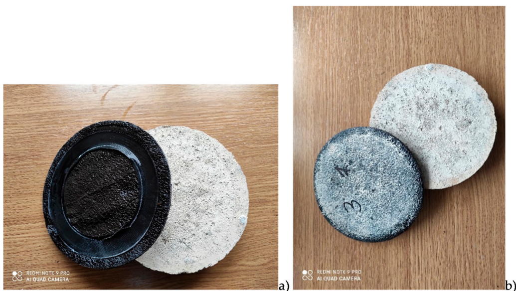
Figure 2. Samples after the waterproofness tests: (a) top side of the sample after removal from the concrete substrate, (b) bottom side of the sample. Next to it, there is a concrete substrate.
