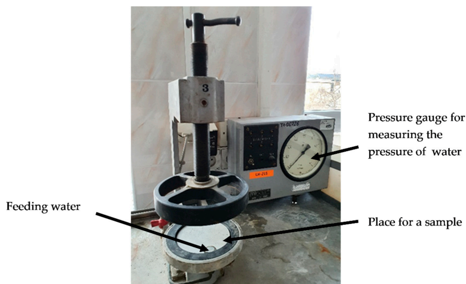
Figure 1. Equipment for testing water absorption of coatings.
