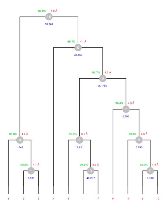
Figure 6. Annotated dendrogram for the 11 datasets used from the serial group 2. Each numbered node corresponds to a cluster Around each node there are three values annotated with overall completeness (green), resolution as computed using  $CC_{1/2}$  (red) and overall Rmeas (blue).
