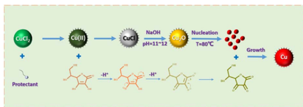
Fig. 10 Mechanism of formation of the ultrafine Cu powder particles.
