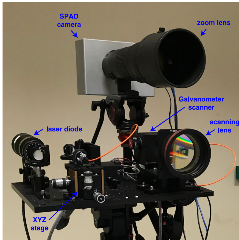
Figure 5. Photograph of the scanning pulsed illumination system and SPAD camera.
