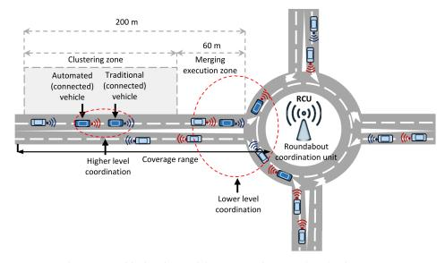
**Figure 1.** The proposed bi-level roundabout control system (RCS). The environment contains automated and traditional connected vehicles. The RCU has two-way communication facility and coordinates automated vehicles at the higher and lower levels.
