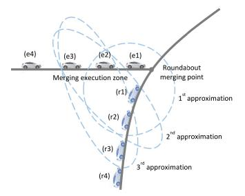
**Figure 4.** Successive optimization of vehicles (blue dashed regions) in a receding horizon approach in the lower level coordination.
