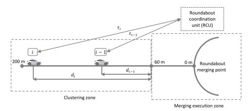
**Figure 3.** Illustration of the principle to determine the necessity of forming vehicle clusters (higher level coordination). The RCU computes the optimal arrival time of vehicles i - 1 and i.
