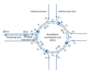
Figure 2. Traffic flow diagram (TFD) of a single-lane four-legged roundabout.
