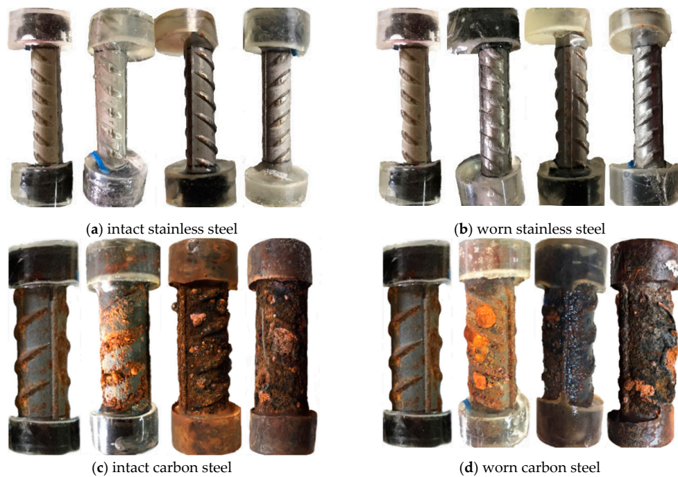
Figure 12. Corrosion state of intact and worn stainless and carbon steels after 0, 10, 90 and 160 days' exposure.
