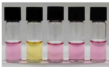
FIGURE 4 | Visual selectivity test of NAz-6-Bpin in THF (0.5 mM) and halide analyte, 1:1. From left to right: no analyte, TBAF, TBACl, TBABr, TBAI. Photo taken immediately after addition of TBAX salt.
