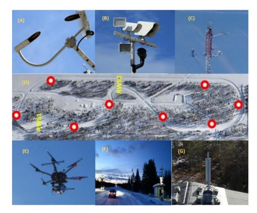
**Figure 5.** (**A**) Visibility and weather detector; (**B**) surface state sensor; (**C**) road weather station and camera; (**D**) test track; (**E**) test track equipped with IoT sensors (i.e., red spots); (**E**) drone; (**F**) field measurements in a real environment; (**G**) 5GTN road weather stations.
