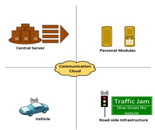
Figure 2. C-ITS architecture communication modules.
