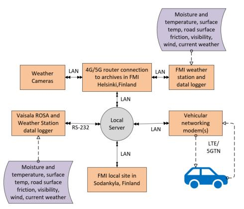
temperature sensor data; vehicle telematics data using CAN bus. For the V2I scenarios, a vehicle was used to interact with the two RWS while passing them on the test track.
