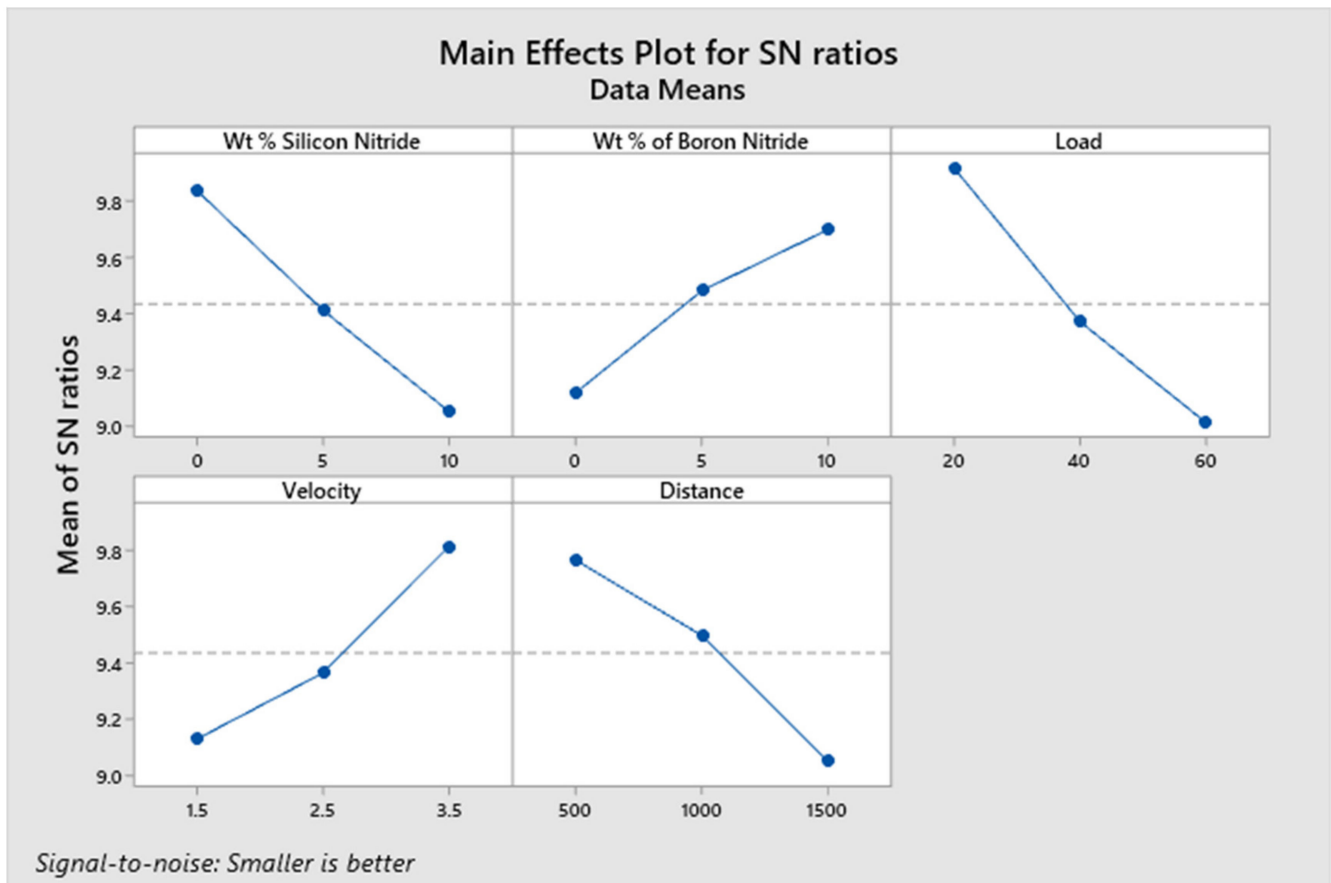
Figure 5. Effect of independent process parameters on COF.
