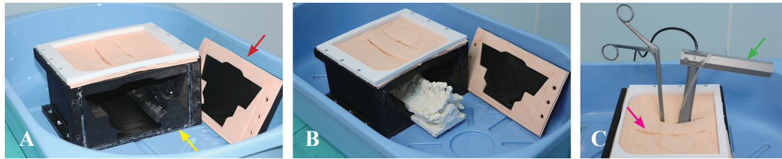
Fig. 2. The training model housing and setup. (A) The dark chamber with sliding mechanism (yellow arrow) and removable lid with gasket (red arrow). (B) View showing the cervical spine model being inserted into the sliding track of the chamber. (C) The complete setup in surgical configuration, showing the slit openings for instrument access (magenta arrow) and the endoscope with custom handle (green arrow).
