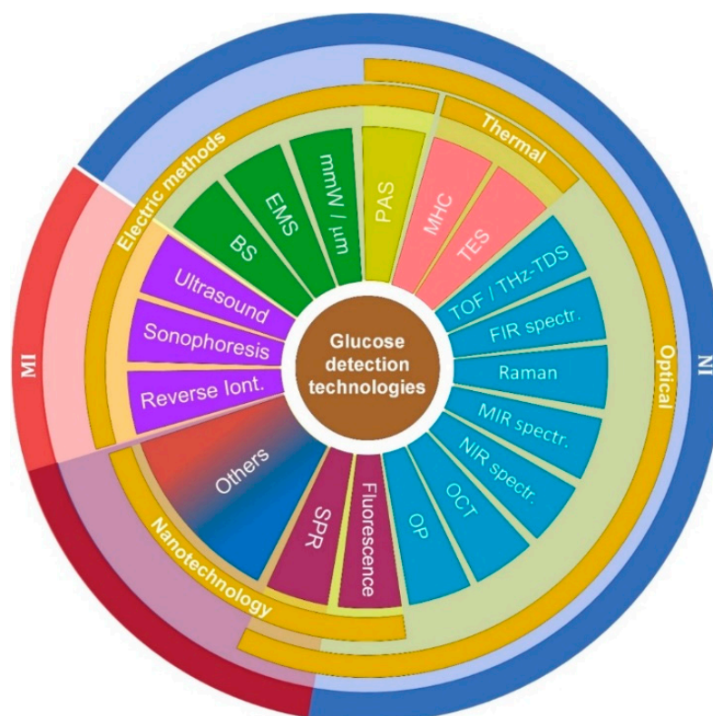
Figure 5. Technologies under development for minimally-invasive and non-invasive glucose detection (SPR-surface plasmon resonance, OP-optical polarimetry, OCT-optical coherence tomography, TOF-time of flight, THz-TDS-Terahertz time domain spectroscopy, TES-thermal spectroscopy, MHC-metabolic heat conformation, PAS-photo-acoustic spectroscopy, mmW-millimeter wave, \mu\text{m} -Microwave, EMS-Electromagnetic sensing, BS-Bioimpedance spectroscopy).
