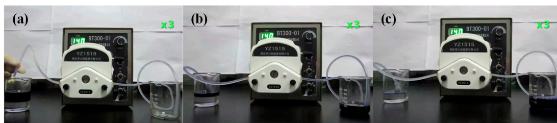
Figure 9. The process of continuous oil/water separation of modified sponge, which was assisted by a peristaltic pump. (a) Before separation; (b) during separation; (c) after separation.
