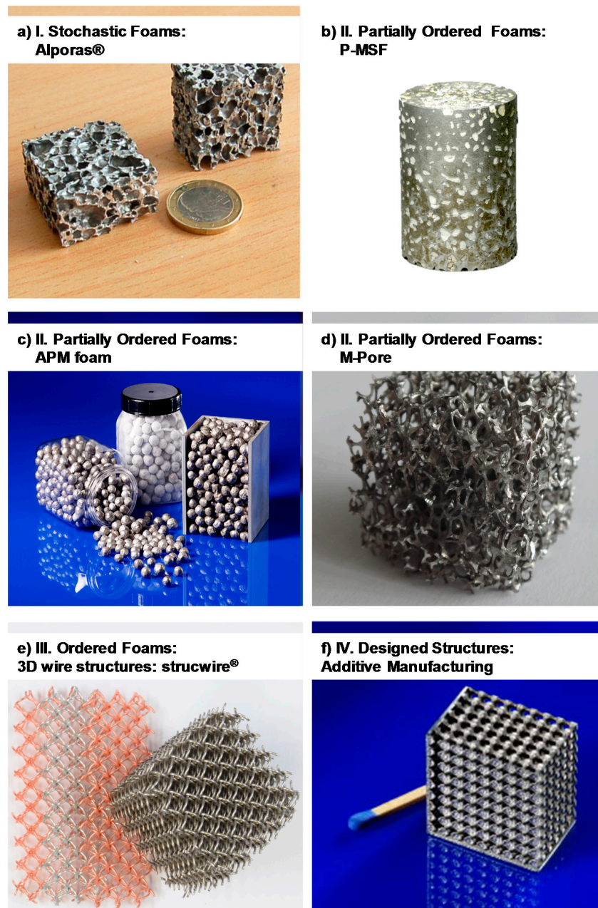
Figure 4. Exemplary images of foam samples representing the four main process categories, illustrating the levels of order and structural control associated with them [79]. (a) Alporas® foam; (b) P-MSF foam; (c) APM foam; (d) M-Pore foam; (e) strucwire® 3D wire structure; (f) additively manufactured 3D lattice structure.
