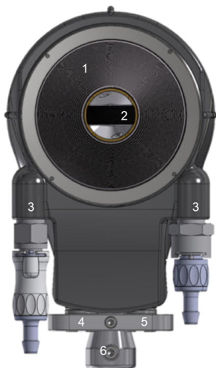
Figure 1. Schematic of the HIFU intraoperative device. 1: HIFU transducer divided into 32 concentric rings. 2: Ultrasound imaging probe. 3: Connectors for the cooling circuit. 4: Connectors for the coaxial cables of the HIFU emitters. 5: Connectors for the cables of the ultrasound imaging probe. 6: Connector for the mechanical arm.
