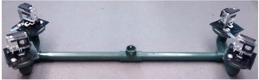
FIGURE 2 Camera head consisting of four GoPro underwater video cameras, mounted in pairs with overlapping fields of view to allow three-dimensional reconstructions of fish swimming trajectories
