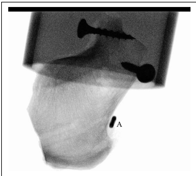
Figure 2. Samples were imaged using fluoroscopy. All specimens underwent bone density analysis following interference screw or interference screw and cortical button placement (A). Specimens were placed on the scanning platform with the medial side facing upward and scanned with a 55-kV C-arm (FluorSCAN InSight FD, Hologic).
