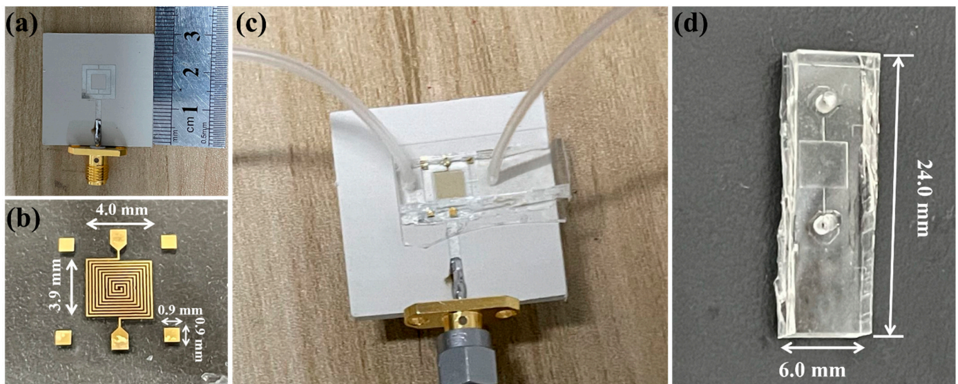
Figure 3. The fabricated RFID chip, including (a) Reader, (b) Tag, (c) RFID chip, and (d) microchannel.
