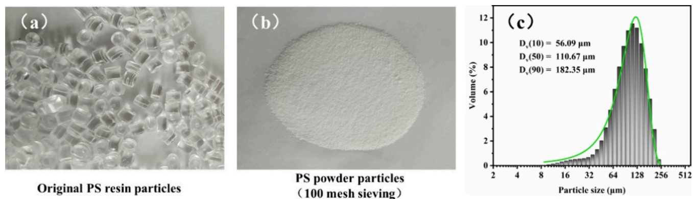
Figure 1. Schematic diagram of a granular PS solid resin sample (a), schematic diagram of a powdered PS sample (100 mesh) (b), and particle size distribution of PS powder after sieving (c).
