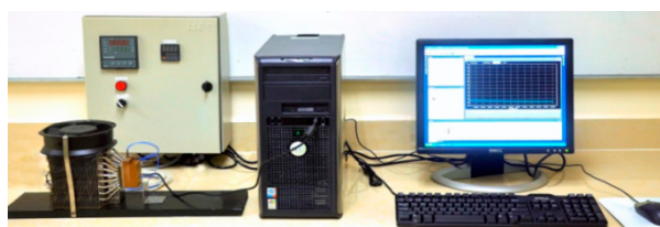
Figure 1. In-house thermal cycling test system.
