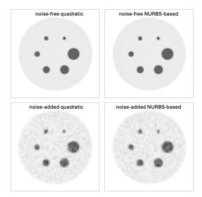
Figure 6: Time-of-flight reconstructions of test object 1 made with Duetto in MATLAB using settings for a Dicovery MI 3-ring PET/CT scanner. Noisy coincidences in the final simulations were: 17.6M prompts, 4.0M randoms, 3.7M scatters.
