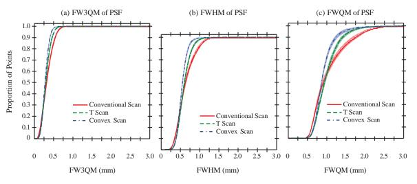
Figure 6. Blurring in the z direction is mitigated by the convex scanning motion as illustrated by three PSF width measures.
