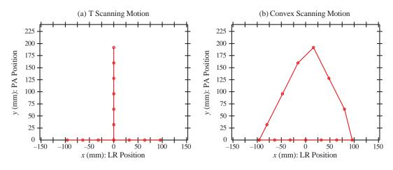
Figure 2. The NGT system supports PA motion unlike current clinical DBT systems. Two simulated motions are shown.
