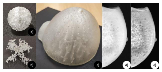
Figure 6. Printed physical models of the (a) spheres, (b) tumor entity and (c) shape, as well as the (d) unprocessed and (e) processed X-ray mammography projections of the phantom.
