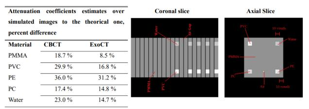
**Table I**. Percent difference between attenuation coefficients estimated in-silico and the theoretical ones at the central axial plane of the FOV. In the ExoCT, 4 projections per oscillations were adopted for 300 oscillations; in CBCT 300 projections were adopted. On the right, a schematic of the used digital phantom.
