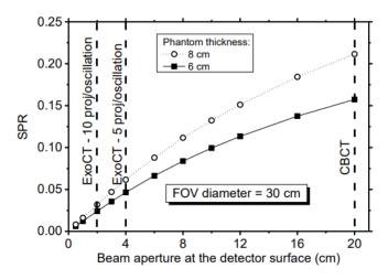
Figure 1. Scatter-to-primary SPR as function of the beam aperture at the detector surface; the irradiated sample was a 10 cm  $\times$  10 cm box made of soft tissue whose thickness was either 8 cm or 6 cm. Source-to-isocenter distance = 500 mm; source-to-detector distance = 750 mm; W/Al 80 kV spectrum.
