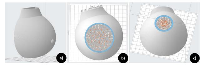
Figure 4. Computational model of (a) the uncompressed breast phantom, (b-c) cross section of the breast model prepared for printing with a slicing software, the supporting structures added inside the model are visible, which were used also to mimic the glandular structures in the breast.
