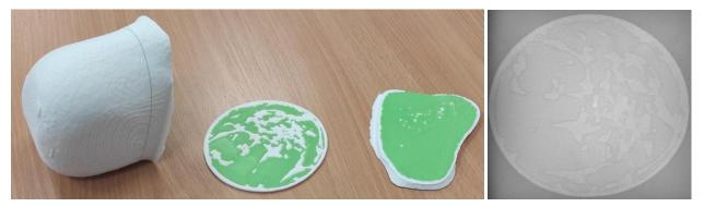
Figure 8. Printed breast phantom and two printed slices. The radiography image on the right is the x-ray image of the slice, shown in the middle.
