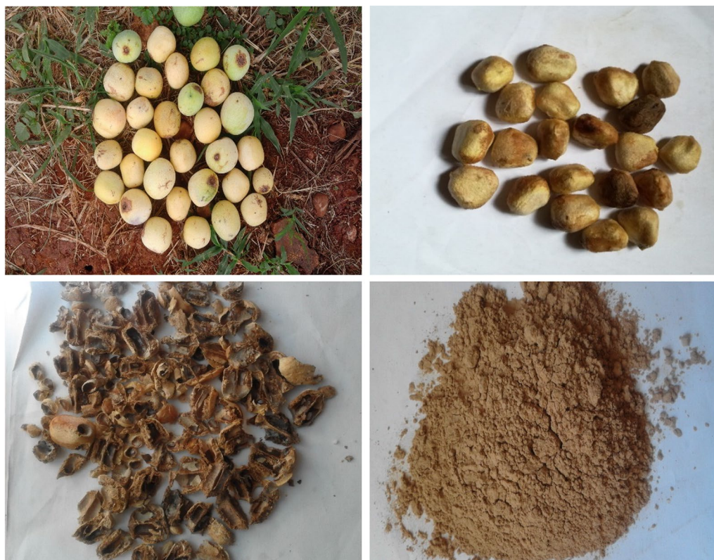
Fig. 1 Stages of adsorbent preparation: top left is the Marula fruits, top right is the Marula seeds, down left is the shell of the Marula seed while down right is the pulverized Marula seed husk
