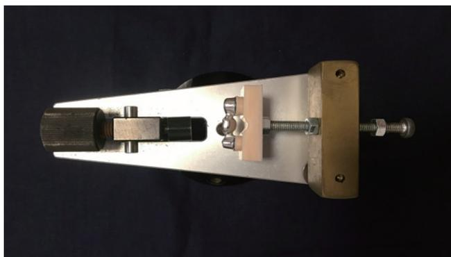
**Fig. 2.** The parallelometer sub-tray stand, which allows rotation of die models, used in marginal discrepancy measurements.
