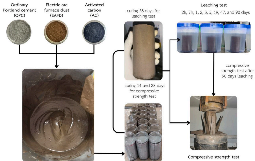
Fig. 1. The procedure for evaluating the compressive strength and leaching characteristics in the immobilization of Cs-137 contaminated Electric Arc Furnace Dust (EAFD).
