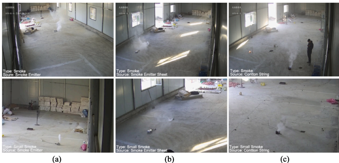
Fig. 3. Self-created grain bins smoke dataset: (a) Smoke Emitter; (b) Smoke Emitter Sheet; (c) Cotton String. The photos are the dataset of smoke in the first row and small smoke in the second row.
