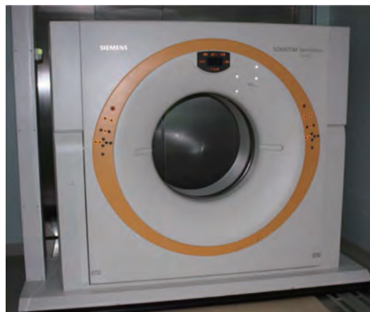
图1 手术室中电子计算机断层扫描 (CT) 设备 Fig 1 Computed tomography (CT) scanner
