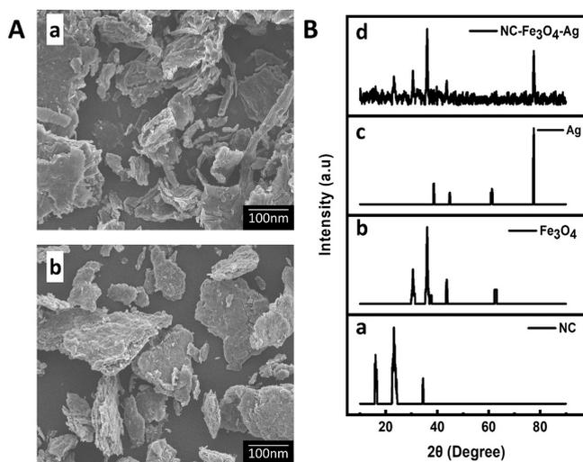
**Figure 2.** (A) SEM micrographs of (a) nanocellulose; (b) NC-Fe<sub>3</sub>O<sub>4</sub>-Ag nanocomposite; (B) XRD pattern of (a) nanocellulose; (b) Fe<sub>3</sub>O<sub>4</sub> NPs; (c) Ag NPs; (d) NC-Fe<sub>3</sub>O<sub>4</sub>-Ag.
