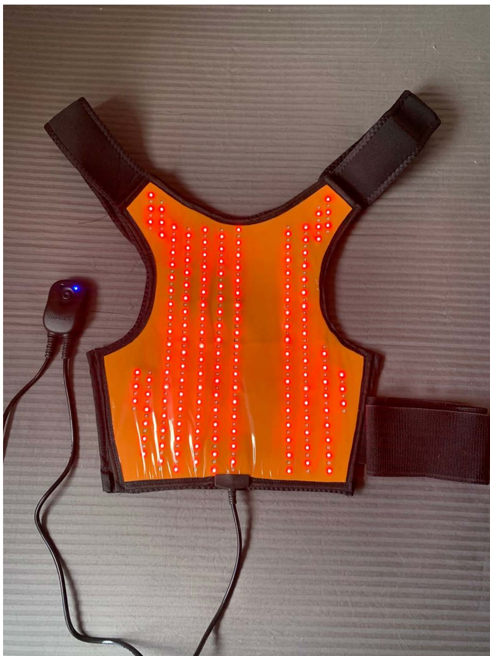
Fig 4. PBM device. Figure 4: Internal view of the activated shoulder pad highlighting the visible red LEDs and the invisible infrared LEDs.
