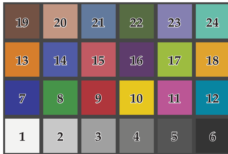
Figure 2. The measured target X-Rite ColorChecker Classic and the patch numbers used in this study.
