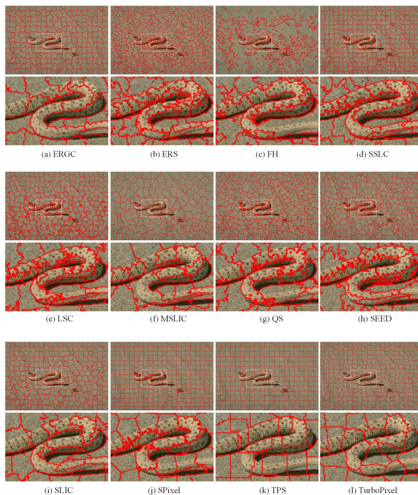
Figure 6. Superpixel segmentations from an image with low variance in color. The first, third and fifth rows are superpixels generated by various methods. The second, fourth and sixth rows zoom in on the regions of interest as defined by the white boxes to facilitate close visual inspection.
