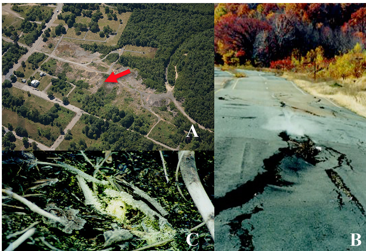
Figure 1. The Centralia, Pennsylvania, mine fire has dramatically impacted the surface environment. (A) Aerial view of the Centralia Mine Fire in July, 2007. Bare ground indicates mine fire-affected sites. The location from which soil samples were collected is indicated by the arrow. (B) Land collapses have caused route 61 in Centralia to crack and buckle, while steam filled with combustion products can be seen rising from the fire below. (C) Elemental sulfur crystals that precipitate at the surface support sulfur-cycling bacteria.
