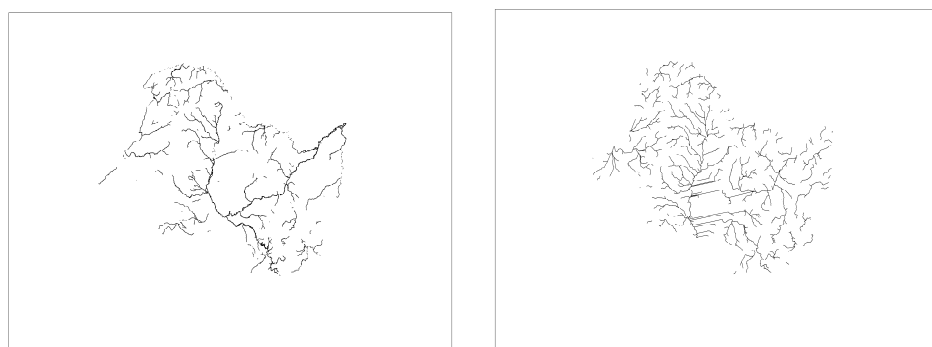
Figure 5. In the SRB, river in land use and the river under the optimal threshold. On the left are the rivers obtained from the land use data. On the right is the river network extracted with the threshold 133,280.
