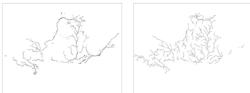
Figure 6. In the YRB, river in land use and the river under the optimal threshold. On the left are the rivers obtained from the land use data. On the right is the river network extracted with the threshold 126,590.
