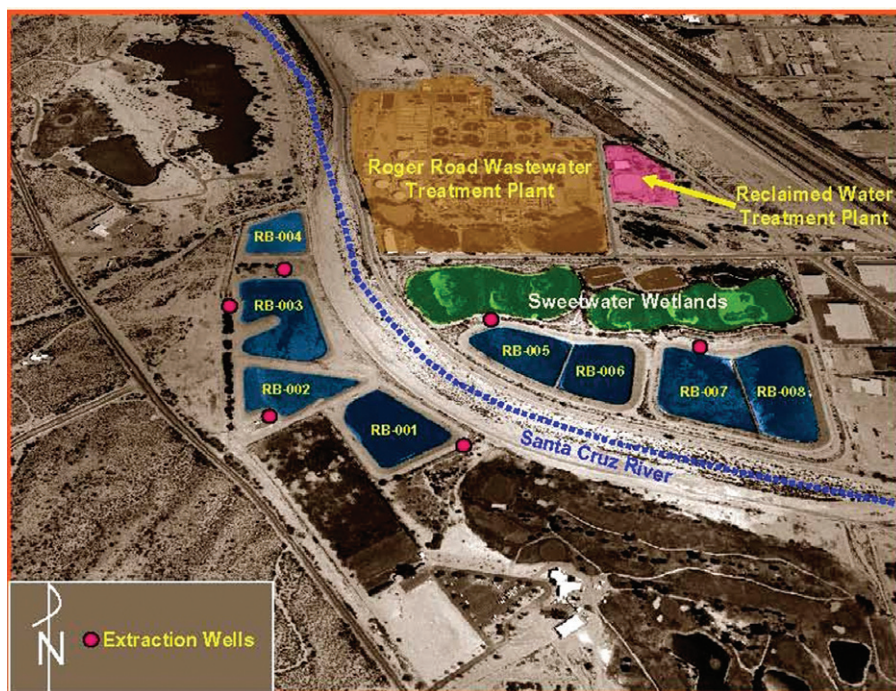
FIGURE 24.22 Aerial view of Sweetwater Recharge Facilities. Numbered blue areas are infiltration basins. Photo courtesy of the Water Reuse Association.
