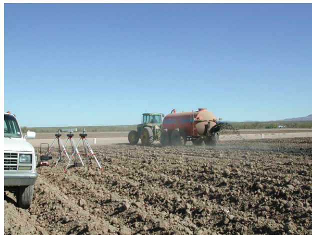
FIGURE 24.28 Land application of liquid biosolids via a spray applicator. Courtesy I. L. Pepper.
