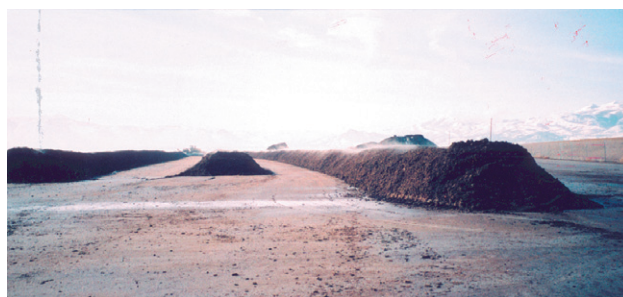
FIGURE 24.27 Biosolid composting via the windrow process. Here three windrows are illustrated. From Pepper, Gerba, and Brusseau, 2006.
