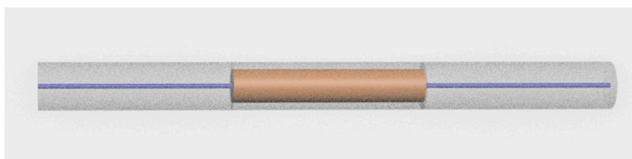
Figure 1. Schematic configuration of an SMS fiber structure [22]. Reproduced with permission from Xianfan Wang, Elfed Lewis, Pengfei Wang, Investigation of the Self-Imaging Position of a Singlemode-Multimode-Singlemode Optical Fiber Structure; published by Wiley Online Library, 2017.
